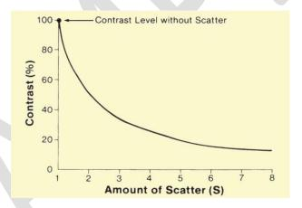
The use of a grid is the most practical method to compensate this loss of contrast. This type of device reduces the scatter radiation that reaches the image receptor. The degree of scatter removing is determined by the Grid Ratio which is the ratio between the heights of the lead strips that make up the grid and their distance.
