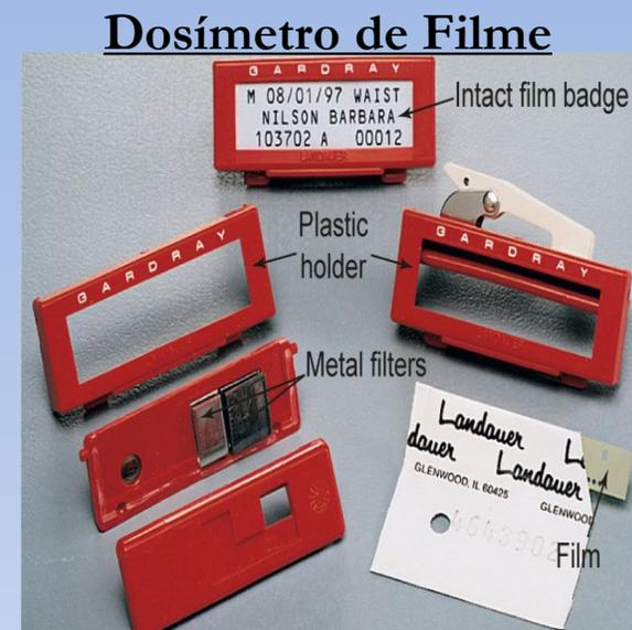
Fig. 5-4. Disassembled film badge, demonstrating badge components: plastic holder, metal filters, and film packet.
