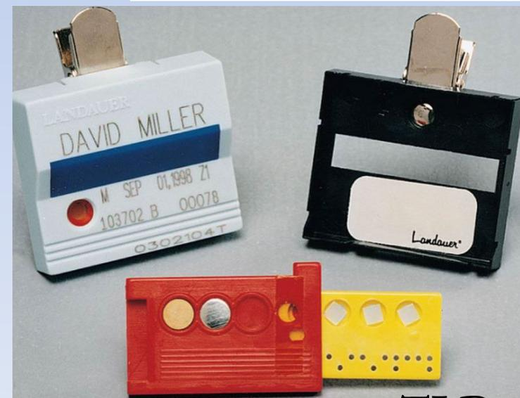
Fig. 5-8. Thermoluminescent dosimeter (TLD) containing the sensing material lithium fluoride (LiF).
