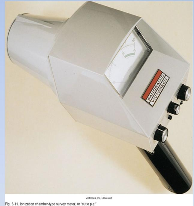
Fig. 5-11. Ionization chamber-type survey meter, or "cutie pie."
